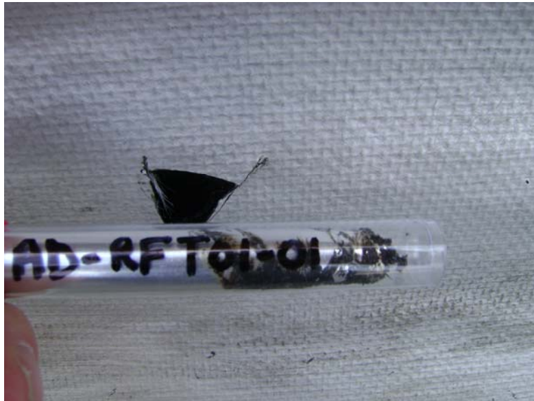
Photo 4 – View of roofing tar and felt containing 20 % and 10% Chrysotile respectively.
